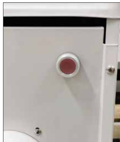
Press and hold the reverse button if the hatches don't close properly.
